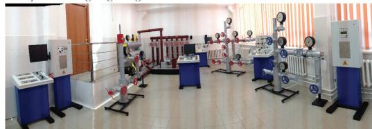
The simulator helps to attain and improve practical skills of performance of main process operations and compliance with safety on production and injection wells, identification and prevention of complications and accidents, well surveillance. The hardware and software of the system submerge the trainee in the situation of a
